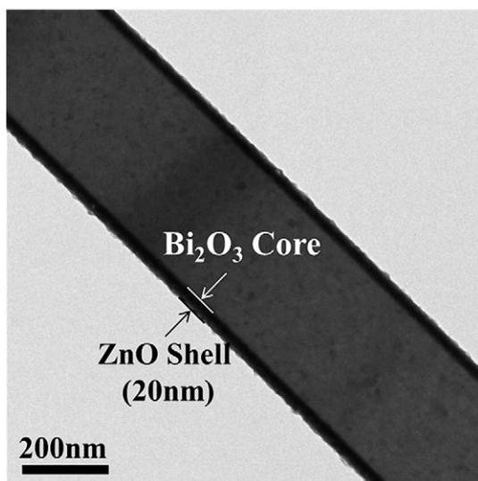
Fig. 3. TEM image of a typical  $\text{Bi}_2\text{O}_3$ -core/ZnO-shell nanobelt.
