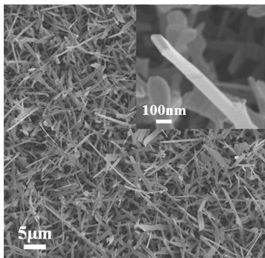
Fig. 1. (a) SEM image of the  $Bi_2O_3$ -core/ZnO-shell nanobelts. Inset, enlarged SEM image of a typical  $Bi_2O_3$ -core/ZnO-shell nanobelt.
