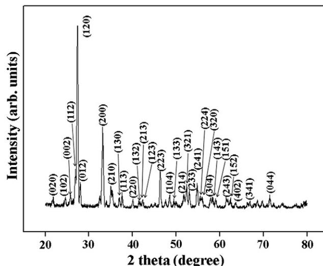
Fig. 2. XRD pattern of the  $Bi_2O_3$ -core/ZnO-shell nanobelts.
