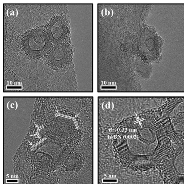
**Fig. 1.** (a,b,c) TEM images of typical *h*-BN fullerenes. In (c), we marked polyhedral shapes and corners. (d) Lattice-resolved TEM image of representative *h*-BN fullerenes.
